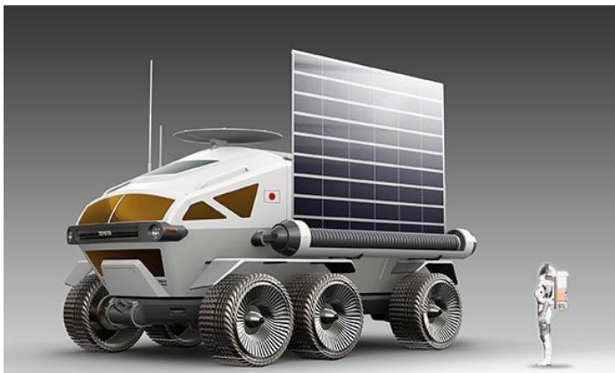
Manned, pressurized rover required for lunar surface mobility Courtesy of Toyota Motor Corporation
