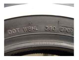
(4) If the white stripe side of the tire is mounted to the inside, check the tires DOT serial number on the black sidewall. If the tire DOT serial number matches any of the following serial numbers,
