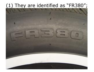
(2) The following information is molded into the sidewall of the tire below the "FR380" marking near the rim: "P235/75R15 105S". If any other size, such as P20575R15 is marked on the sidewall, your tire is not included in this recall.
